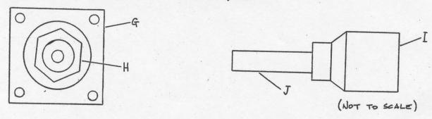
5) The seal parts are now exposed and can be eased out of place. Please note the order of the parts on the drawing below. Order and orientation are important for correct operation.
